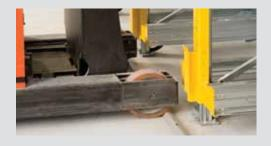
Protective Floor Rail – Protects the rack from collision with the forklift.
