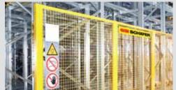
Docking Station – Central safety element with hazard warning light and status display. Prevents unauthorized entry into the aisle. Provides safe transportation of Orbiters.
