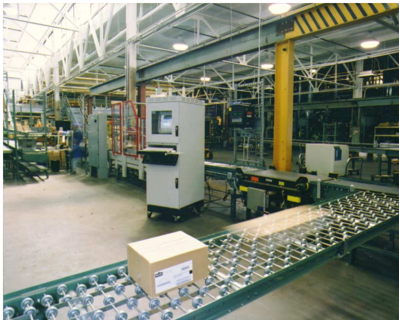
FloStor's material handling installation at Peet's Coffee & Tea (control station at center)
