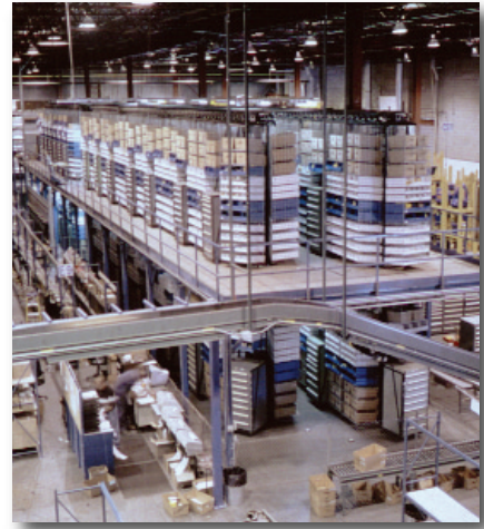
The carousel system is dual tiered on mezzanine to minimize floor space requirements and maximize vertical storage cube.
