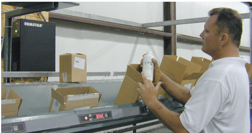
One operator averages 450 to 500 lines per hour and the carousels flexibility allows a second operator to be added to hit 700 lines per hour to meet peak demand with 99.82% accuracy levels.
