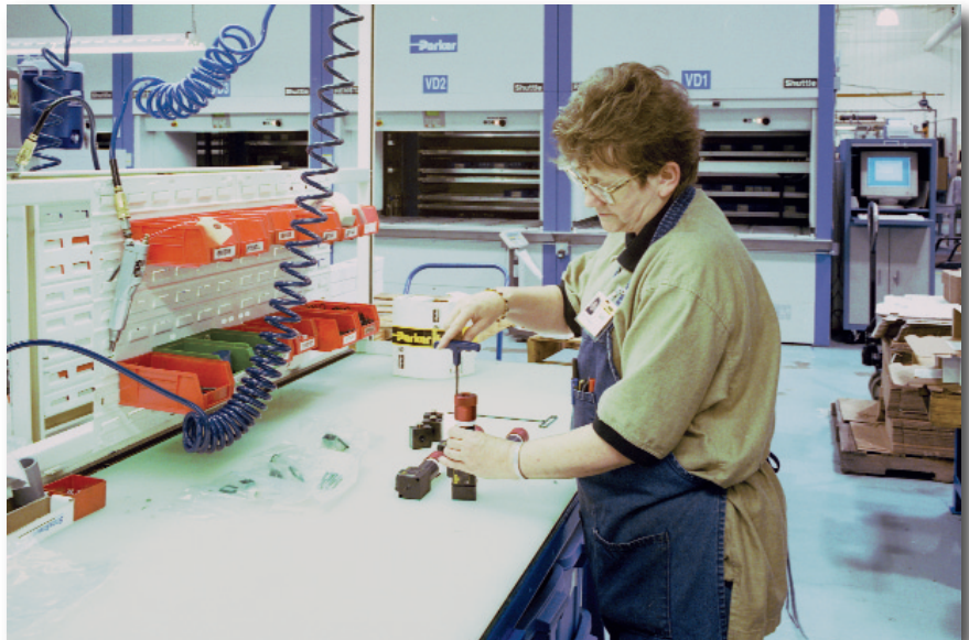
A group of Shuttle VLMs service each work cell. Each cell typically consists of machine tools, assembly tables, and test stands. All orders are manufactured to customer order only to meet 1, 2, or 3 day shipment requirements.
