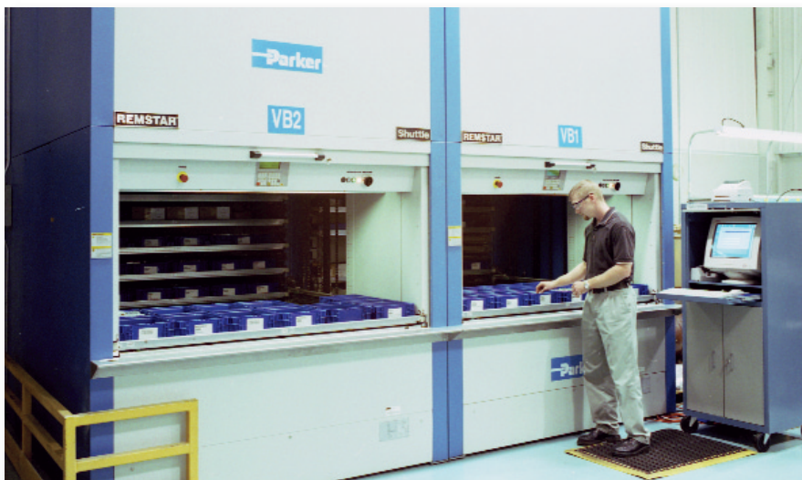
The computer terminals are integrated with FastPic inventory management software. If parts are located in several VLMs keying the single BoM or order number triggers the VLMs to deliver all the parts in sequence.
